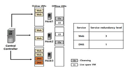
Fig. 8: An example of a conventional SCIT applied in Fig. 7
