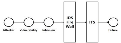
Fig. 2: The concept of Intrusion Tolerance System (ITS)
