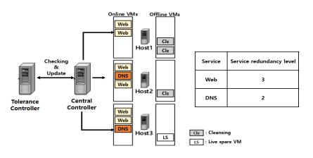
Fig. 9: An example of the proposed scheme applied in Fig. 7
